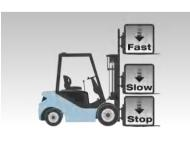
With intelligently declining buffer sensor on the two ends of the cylinder, the falling speed of the fork slows down automatically before it is 10cm from the ground, and the lifting speed to the top also slows down to avoid quick hit on the top, it super increases the safety of the goods and forklifts.
